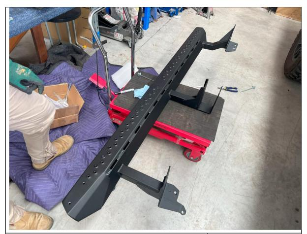
12. Unpack welded slider assembly and position on lifting trolley such that mounts sit approximately level.
